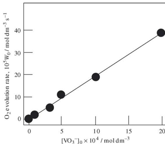
Fig. 1. Plot of initial rate of dioxygen evolution in the H<sub>2</sub>O<sub>2</sub> decomposition in MeCN vs. initial concentration of *n*-Bu<sub>4</sub>NVO<sub>3</sub>. Conditions: [H<sub>2</sub>O<sub>2</sub>]<sub>0</sub> = 0.96 mol dm<sup>-3</sup>; [PCA]<sub>0</sub> = 25 × 10<sup>-4</sup> mol dm<sup>-3</sup>; 50 °C.
