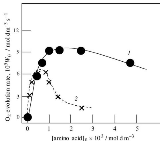
Fig. 3. Plots of initial rate of dioxygen evolution in the  $H_2O_2$  decomposition in MeCN vs. initial concentration of added PCA (curve 1) or picolinic acid (curve 2). Conditions:  $[n\text{-Bu}_4\text{NVO}_3]_0 = 5 \times 10^{-4} \text{ mol dm}^{-3}$ ;  $[H_2O_2]_0 = 0.96 \text{ mol dm}^{-3}$ ;  $50^\circ\text{C}$ .
