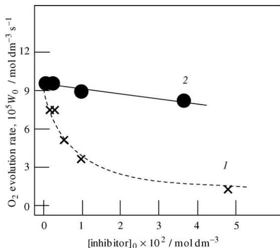
Fig. 5. Plots of initial rate of dioxygen evolution in the  $\text{H}_2\text{O}_2$  decomposition in MeCN vs. initial concentration of added phenol (curve 1) or 2,6-dimethyl-4-*tert*-butylphenol (curve 2). Conditions:  $[\textit{n}\text{-Bu}_4\text{NVO}_3]_0 = 5 \times 10^{-4} \text{ mol dm}^{-3}$ ;  $[\text{PCA}]_0 = 25 \times 10^{-4} \text{ mol dm}^{-3}$ ,  $[\text{H}_2\text{O}_2]_0 = 0.96 \text{ mol dm}^{-3}$ ;  $50^\circ\text{C}$ .
