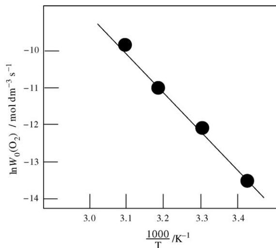
Fig. 4. Dependence of the initial dioxygen evolution rate on temperature in the  $H_2O_2$  decomposition in MeCN which corresponds to  $E_a = 20 \text{ kcal mol}^{-1}$ . Conditions:  $[n\text{-Bu}_4\text{NVO}_3]_0 = 1 \times 10^{-4} \text{ mol dm}^{-3}$ ;  $[\text{PCA}]_0 = 5 \times 10^{-4} \text{ mol dm}^{-3}$ ;  $[H_2O_2]_0 = 0.96 \text{ mol dm}^{-3}$ .
